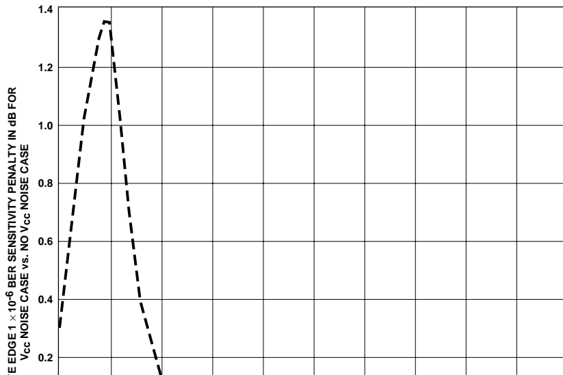
Figure 12. HFBR-510X/520X 1300 nm susceptibility for ≈ 20 V/m fields. 820 nm HFBR-5104/5203 susceptibility plots are not included here, but are as good or better than 1300 nm to within measurement noise (max noise = 0.05dB).
